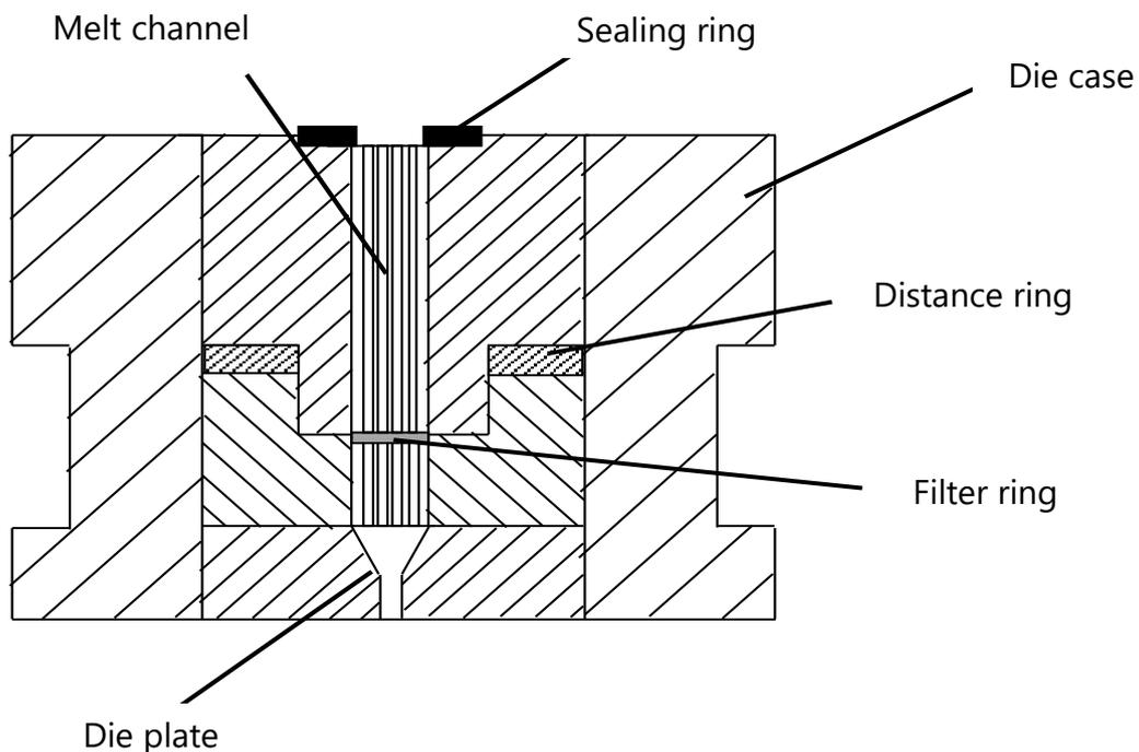
Figure 1. Die set-up for a mechanical and thermal homogenization of the melt
